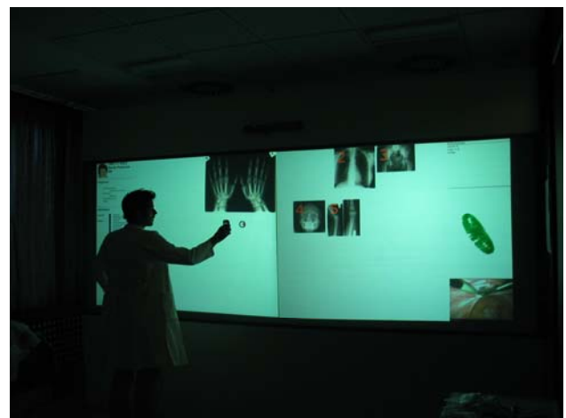
Figure 5: Mixis used to drag, rotate and zoom picture on a large wall display
